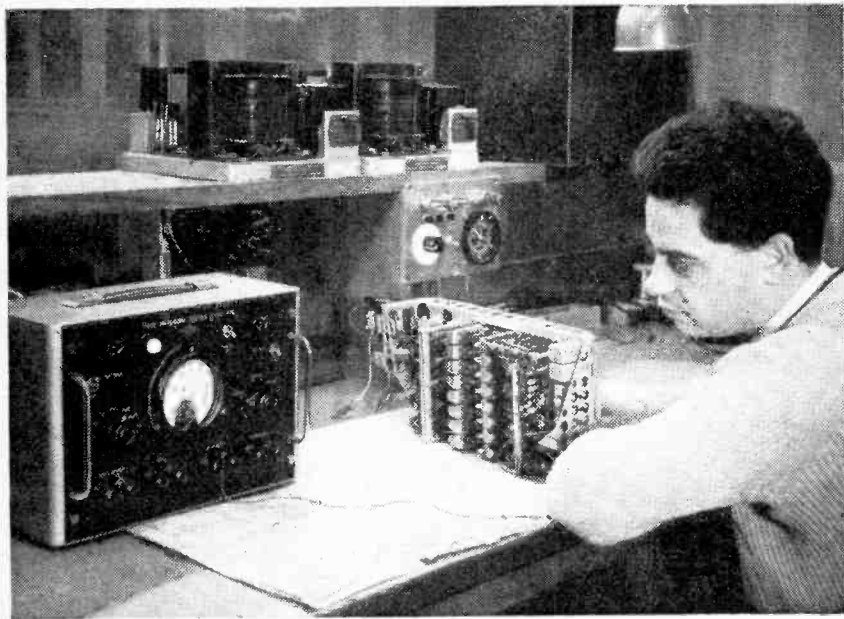
Fig. 5. The timer is also used to check the relay characteristics and timing circuits in the Decca receiver. In this case the Mk 10 lane identification chassis is being timed.
